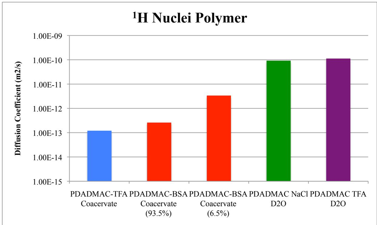
Figure 4: Comparison of diffusion coefficients for  $^1\text{H}$  nuclei of polymer. Blue (left): PDADMAC-TFA-BSA coacervate, Red (second from left): less dense domain of PDADMAC-BSA coacervate, Red (third from left): breaking up of dense domains of PDADMAC-BSA coacervate, Green (second from right): PDADMAC in 0.1M NaCl, Purple (right): PDADMAC-TFA in 0.1 M in sodium trifluoroacetate.
