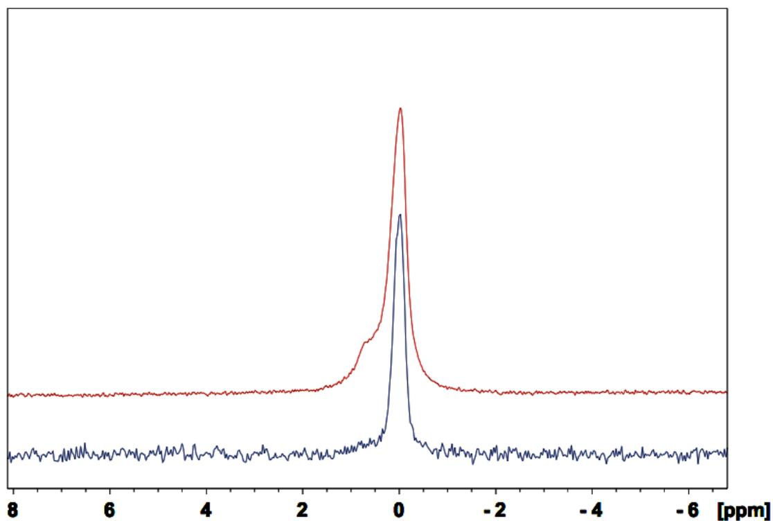
Figure 9: One-dimensional  $^{23}\text{Na}$  NMR spectrum. Red (top): Free-induction decay hinting at a broad component and narrow component. Blue (bottom): PGSTE showing broad component is not measurable.
