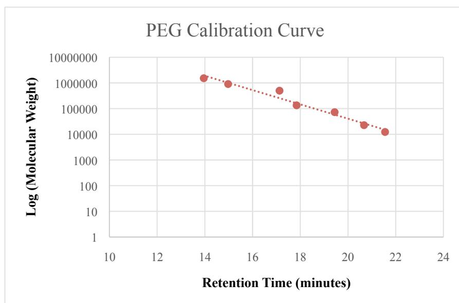
Figure 2: Polyethylene glycol calibration curve with 3<sup>rd</sup> degree polynomial fit. Equation:  $y = -0.014982x^2 + 0.25357x + 5.5569$
