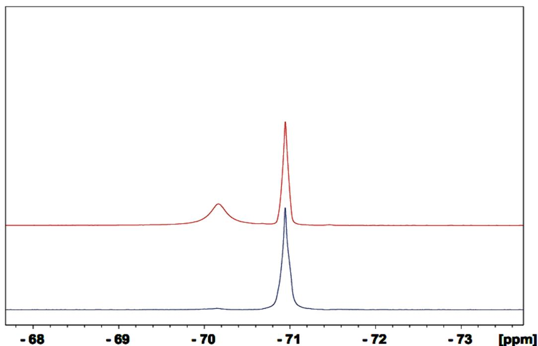
Figure 11: One-dimensional <sup>19</sup>F NMR spectrum. Red (top): Free-induction decay showing two distinct peaks, Blue (bottom): PGSTE showing too fast of relaxation of the nuclear spin state of one of the components.
