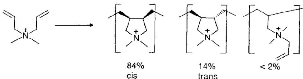
Figure 1: Chemical Structure of PDADMAC via free radical cyclopolymerization [7].
