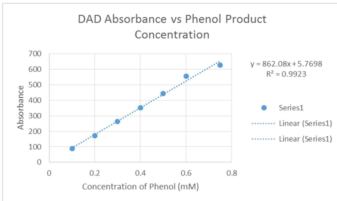
Figure 5: A calibration curve was attained utilizing the phenol standards run under the same methods on the HPLC as the trapping experiment ( $\lambda = 280\text{nm}$ ).
