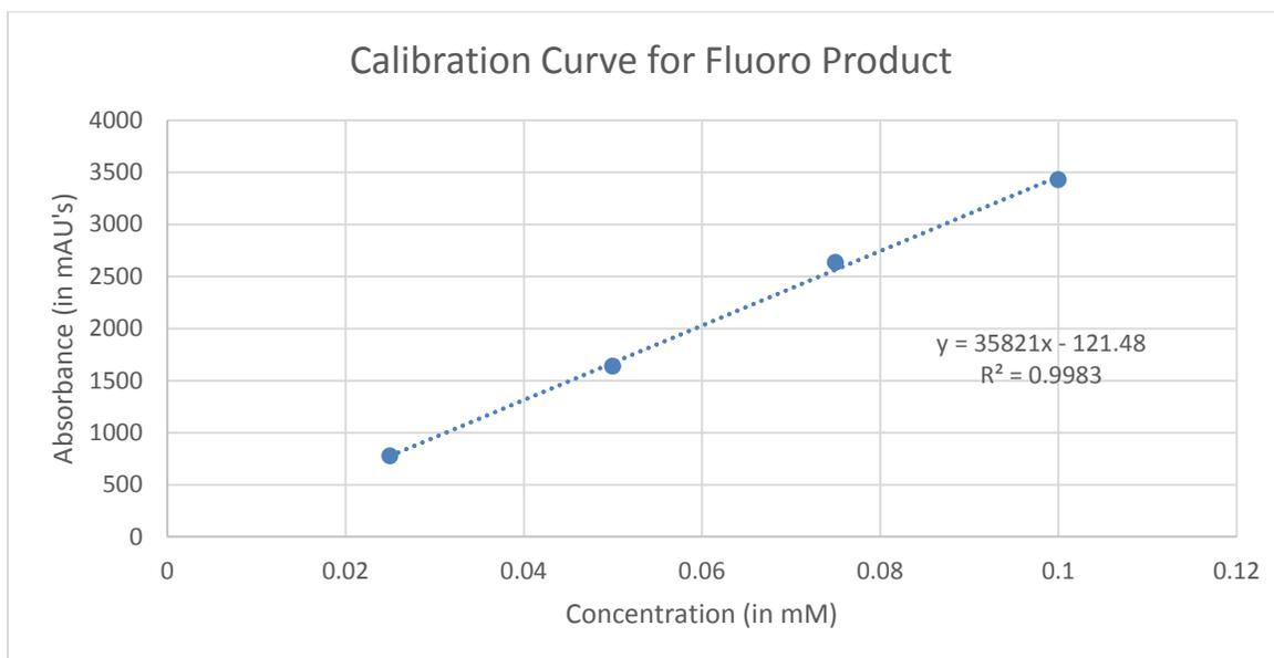
Figure 6: A calibration curve was attained utilizing the phenol standards run under the same methods on the HPLC as the trapping experiment. ( $\lambda = 280\text{nm}$ ).
