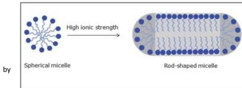
**Figure 1: The addition of salts stabilize the formation of rod-shaped micelles.<sup>K</sup>**
