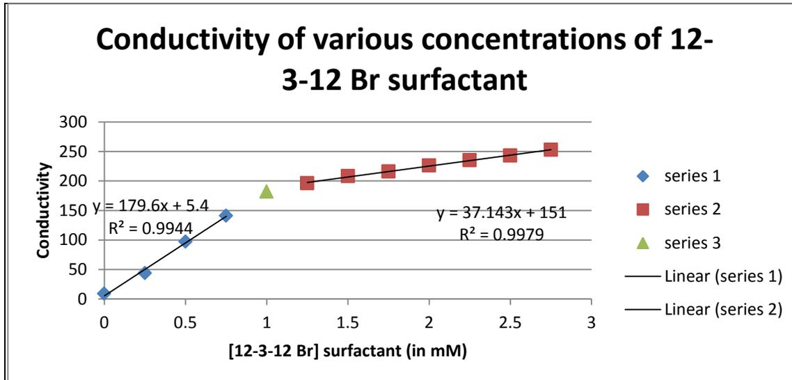
Figure 4: A series of concentrations of 12-3-12 Br surfactant (0-2.75mM) in H<sub>2</sub>O was measured for conductivity in order to determine the CMC.
